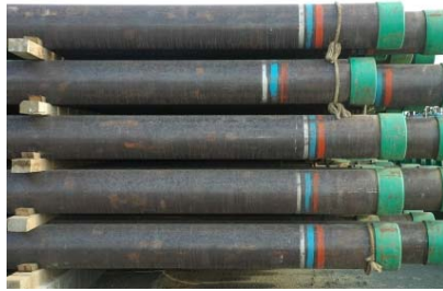
Ductile iron pipe (DIP)
