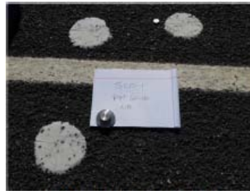
(a) SLO-1 PM 60.16 coarse 3/8" gradation chip seal
