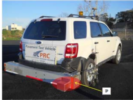
Figure 4.7: Instrumented vehicle with an inertial profiler (IP).
